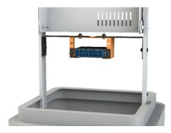
• If there are no existing mounting holes, ensure that the assembled kit is level and mark each post to be drilled. Once marked, drill four .25-inch holes in the mounting posts and attach the assembled bracket kit and magnet mount to the posts using the included 1-inch carriage bolts, flat washers, and M6 hex head bolts. Ensure all hex head bolts are tight to bracket and post as well as to the magnet mount chassis.
